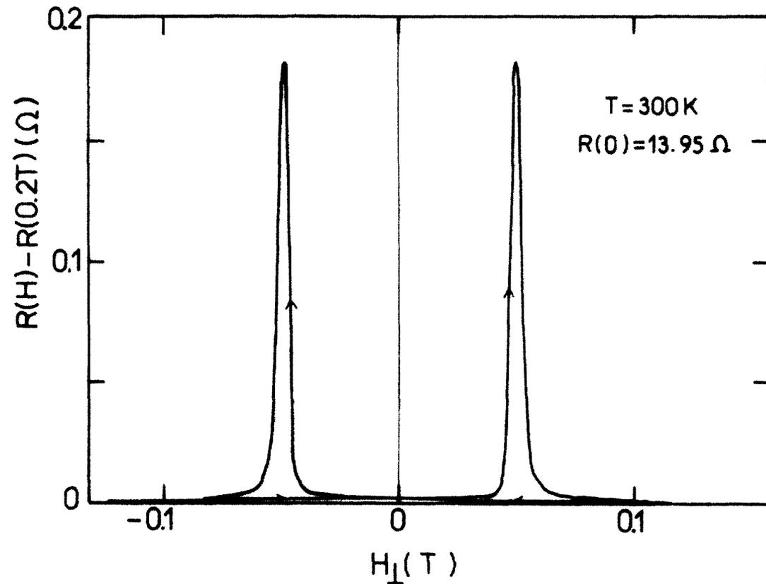
FIG. 3. Room-temperature perpendicular magnetoresistance of sample 3: Au/Co (0.76 nm)/Au (3 nm)/Co (0.76 nm)/Au. The coercive field is  $H_c = 493 \text{ G}$  and  $\delta R_c/R = 1.3\%$ .
