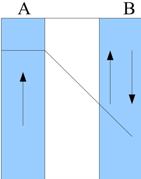
The tunnel rate from A to B through insulator will depend on polarization of B
